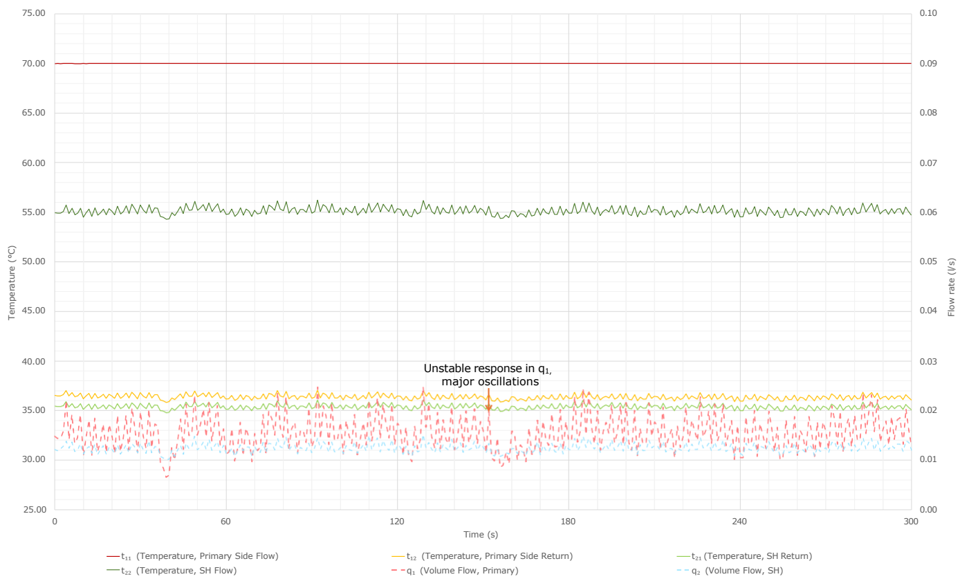
Figure 35 : Example of primary flow rate response for Tests 01a-f for a HIU with less responsive control.
