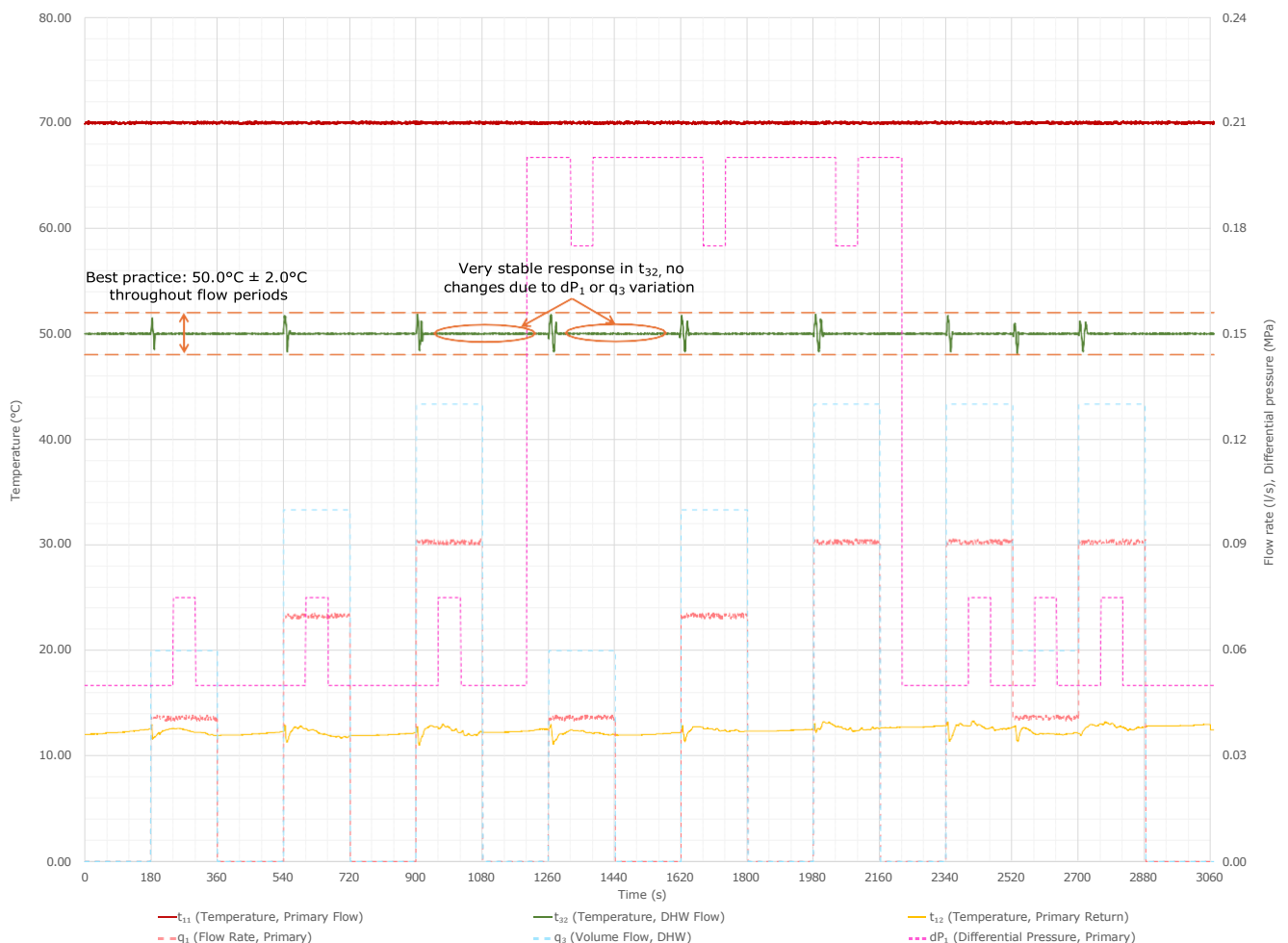
Figure 4 : Example of best practice DHW flow temperature response during Tests 11a-b.
