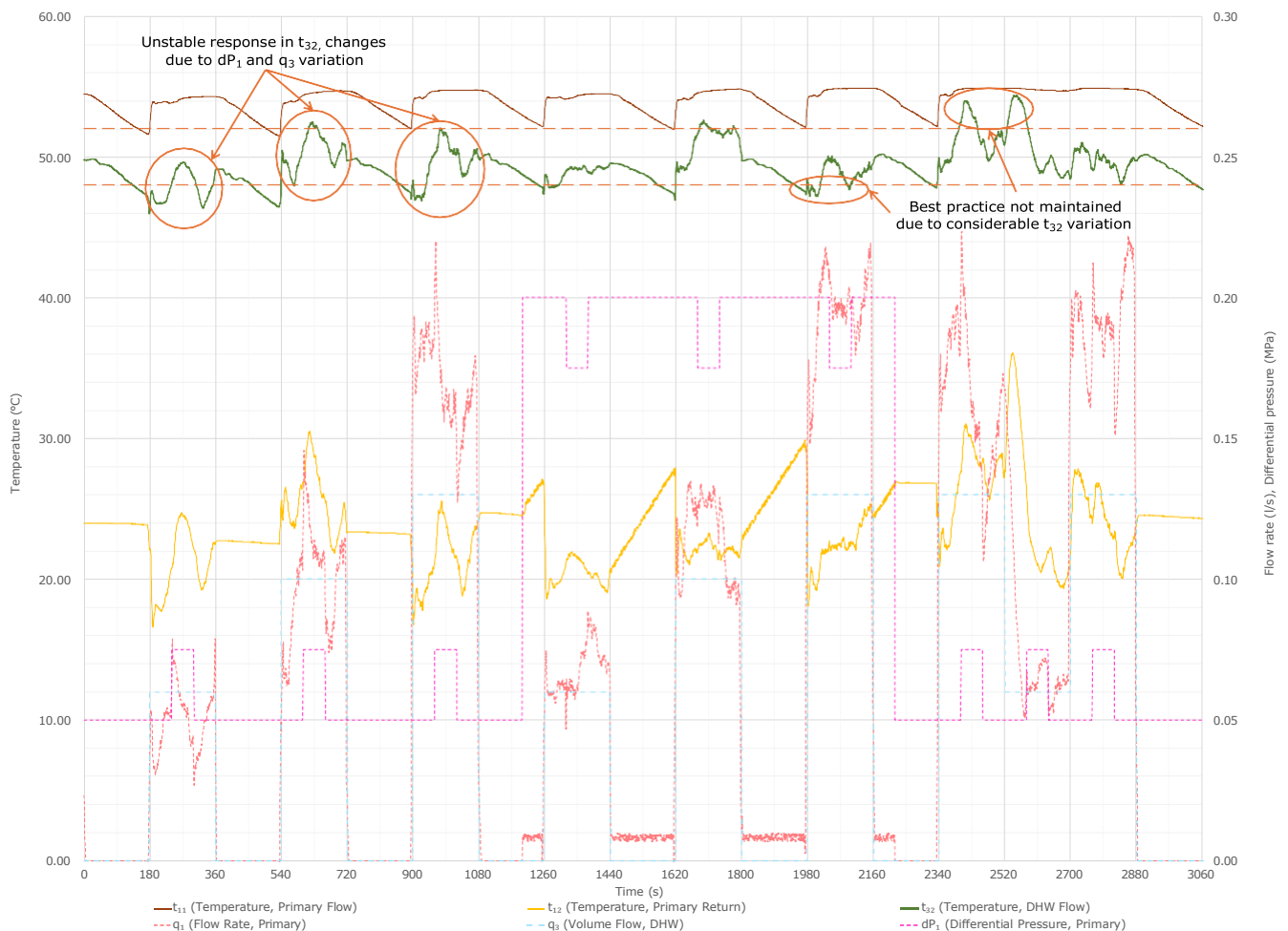
Figure 5 : Example of DHW flow temperature response during Tests 11a-b for a HIU with less responsive control.
