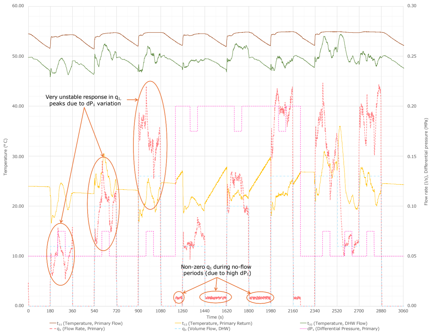
Figure 9 : Example of primary flow rate response during Tests 11a-b for a HIU with less responsive control.
