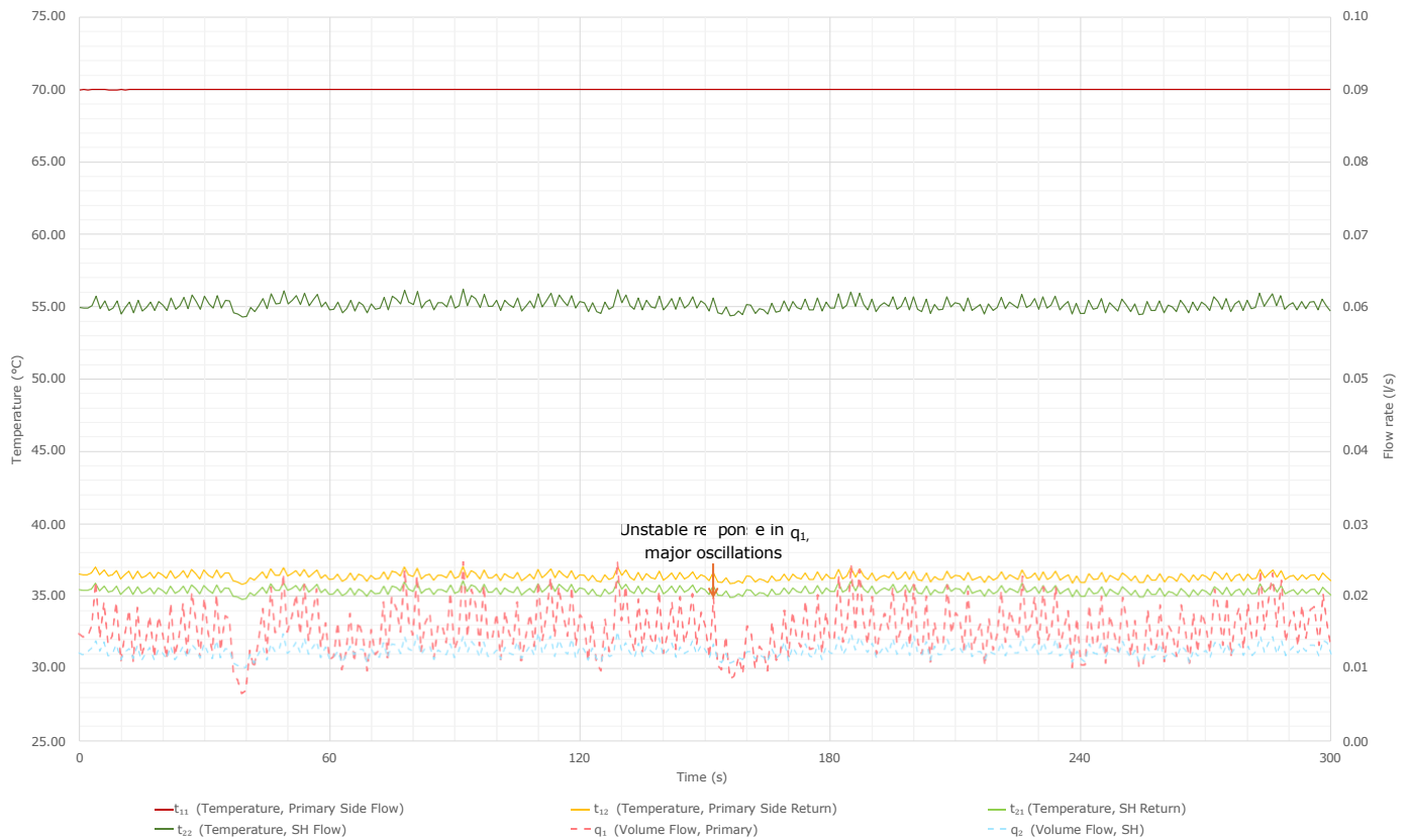
Figure 37 : Example of space heating flow rate response during Tests 01a-f for a HIU with less responsive control.
