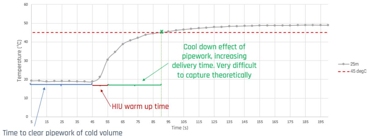
In this case the time for the HIU to *generate* hot water was 10 seconds. Shortening this would not have had a material impact.
