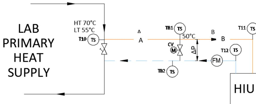
The test setup shall simulate a HIU being located on the 5<sup>th</sup> floor of the vertical riser using the “model scenario”;
