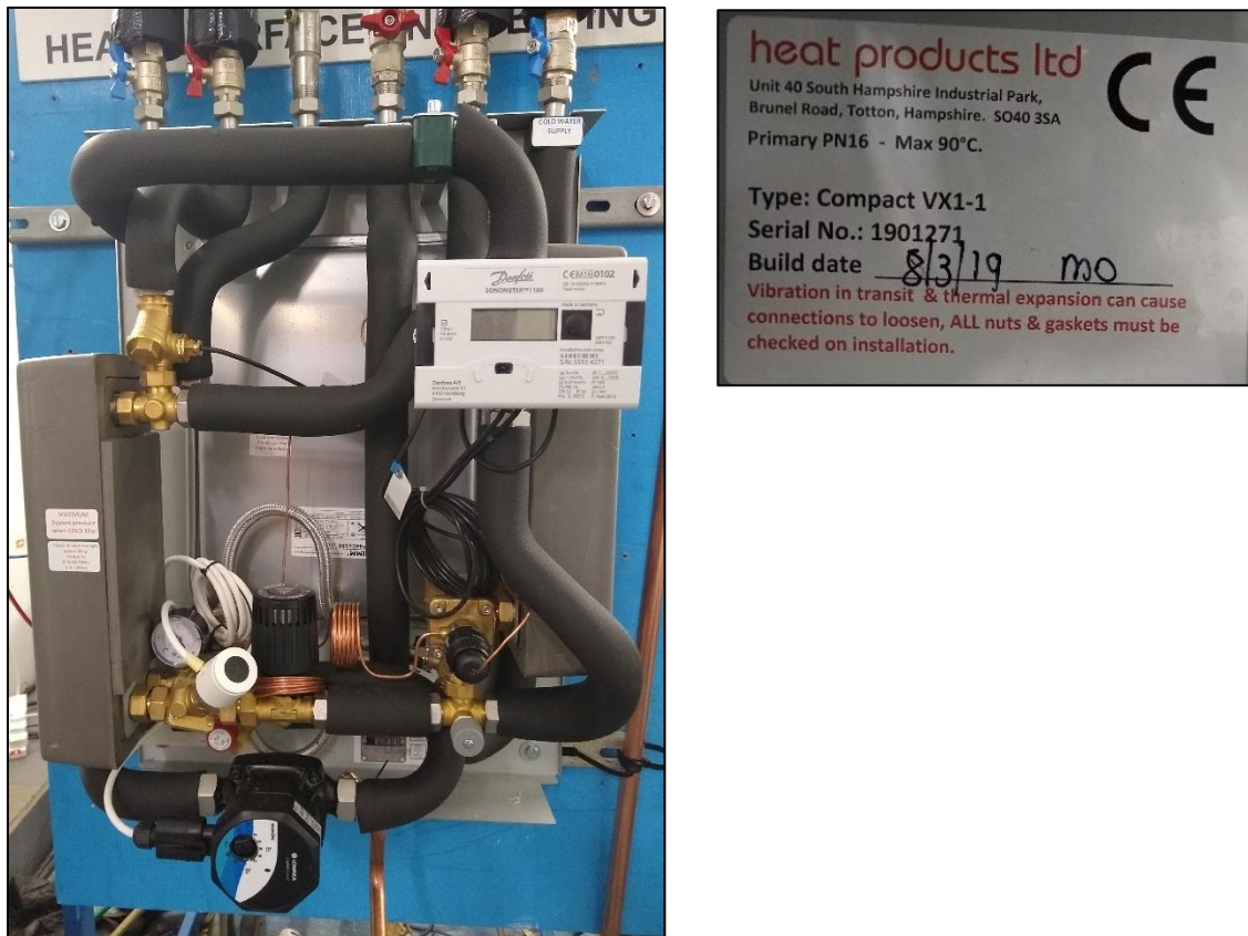
Figure 1 Compact VX1-1 HIU installed in the test rig
