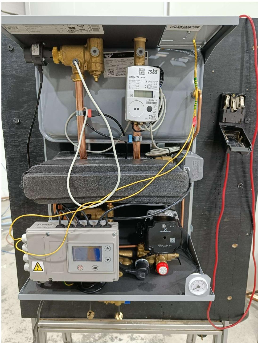
Figure 21 - HIU with Outer Case Removed
