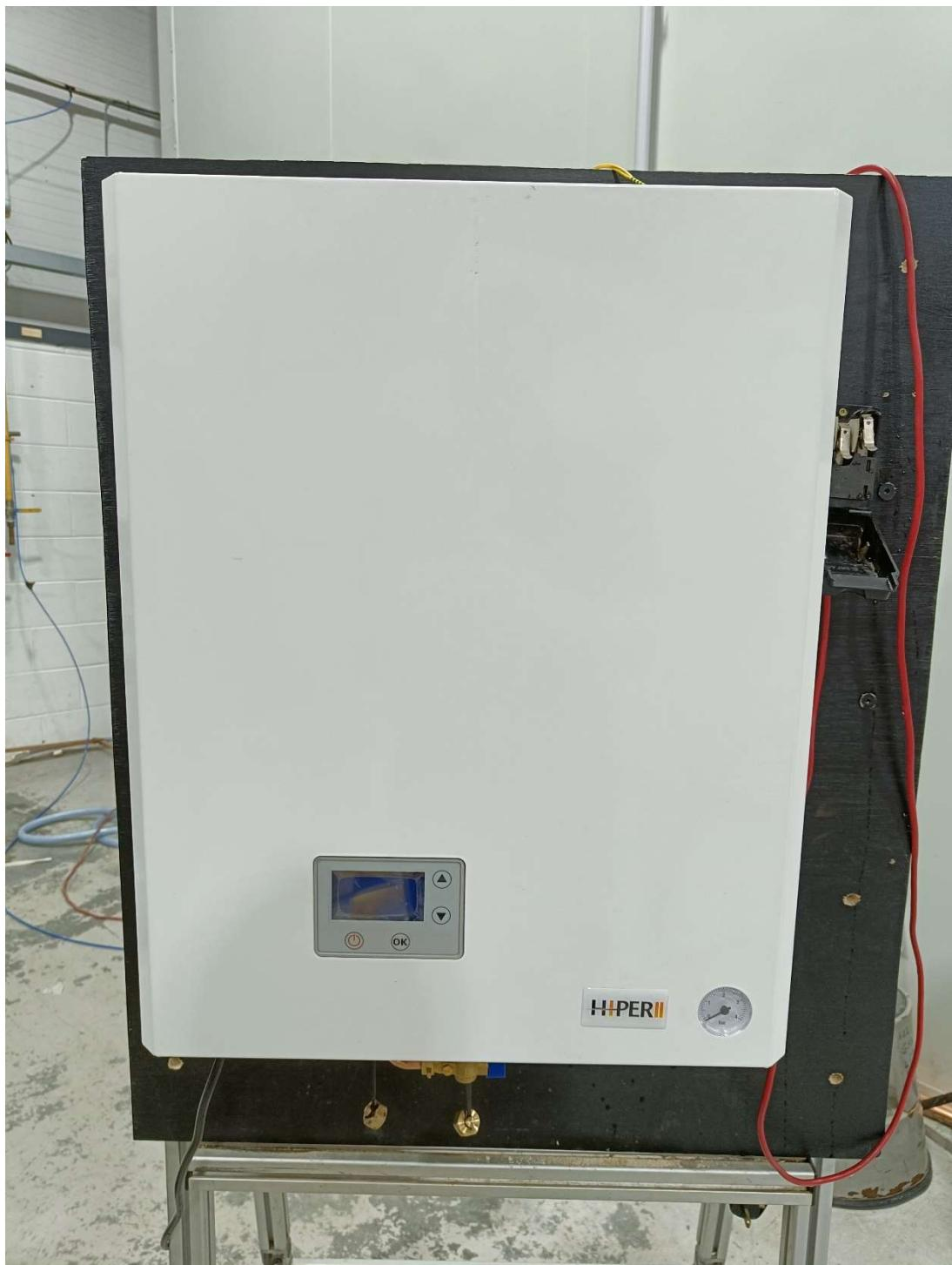
Figure 20 - HIU with Outer Case Fitted
